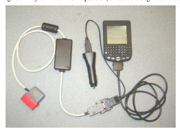
There are a pair of internal DIP switches in the little black box of the OBD2 cable. Turning these switches "ON" will provide enough power to the PDA for scanning, but not for charging. If you use the car charger, you can leave these DIP switches "OFF" (facory default). Turn these switches "ON" if you don't want to use the car charger, or if you are using your own Handspring PDA. If you have a Palm PDA, leave the switches "OFF".
